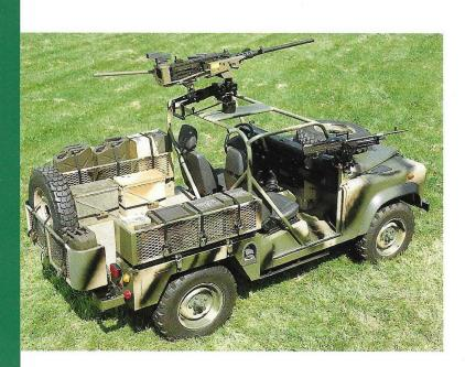
Pedestal mountings can be provided on the front roll cage and at the rear of the vehicle to fire the 0.5 inch Browning, Mk19 40mm grenade launcher and the GIAT 20mm.
