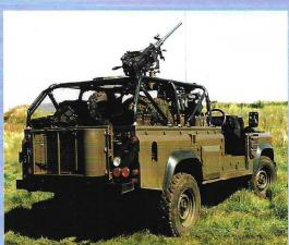
The hinged rear pannier provides additional stowage space (sufficient for spare wheel).
